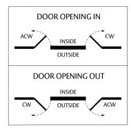
CW (Clockwise) Left Hand open in and Right Hand open out.
